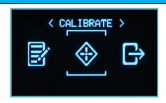
**Calibrate:** Utilize this menu to calibrate the True-D modules for first time usage. It is highly recommended you re-calibrate when using a different video transmitter.
