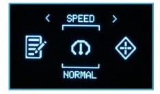
**Speed:** Configure sensitivity and switching speed of filter for the new algorithm. Three choices are available for use:
