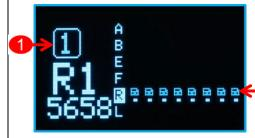
**Saved Channel:** To save channel that you want to choose to start up for the next time and delete undesired channel. When pressing the **Select** button about 3s, you can save/delete/exit. You can save up to 8 channels. The default Saved Channels are R1 to R8.
