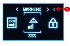
**Warning:** Buzzer will warn you at configured low signal level. The options are as follows: **None, 20%, 35%** and **50%.** If a low signal is detected on antenna A, the buzzer will single beep and if a low signal is detected on antenna B the buzzer will dual beep.
