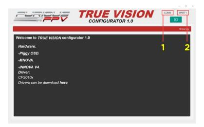
**STEP 4:** Plug Battery for Kombini DS, then click **Connect icon** on True Vision interface to connect and configuration OSD layout and setting.
