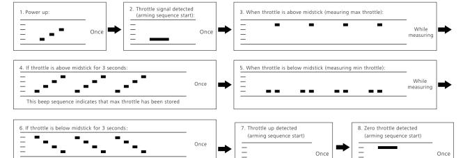
At this point throttle calibration values are stored. You may remove power from the ESC, or just continue running your ESC
