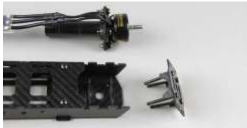
17. Lock the carbon tube with four screws through extruding way.
