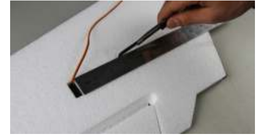
6. Then cut a slot on bottom wing for embedding the servo lead.
