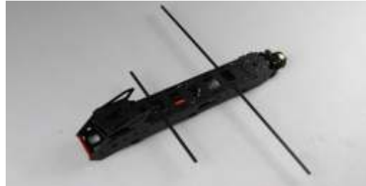
14. Insert the wing reinforcing rod in the fuselage.
