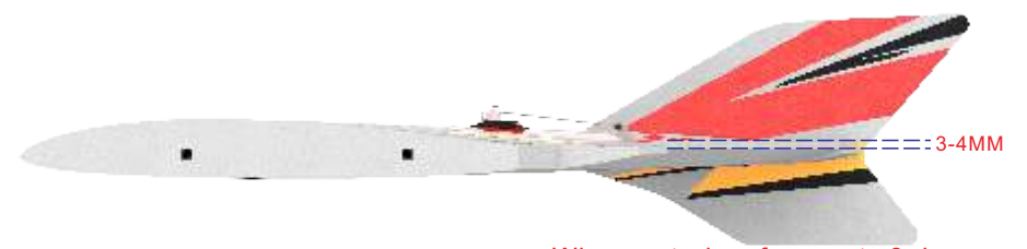
Wing control surface up to 3-4mm
