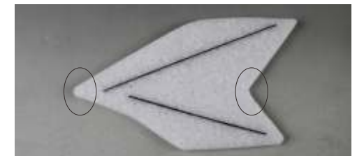
12. The pointed position in black circle is the adhesive position of wing fence, which would be glued on the wingtip.
