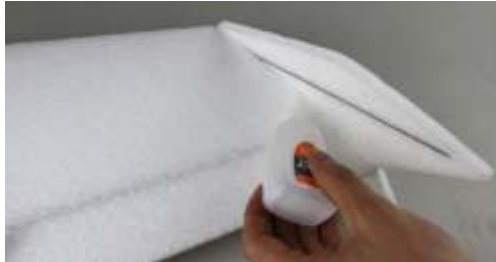
13. Install wing fences on wing tips position with glue.
