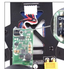
Dipswitch on the transmitter
