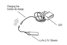
Please switch on the remote control, insert the charge plug into the E728 insert the Li-Po battery into the charge plug as the picture showed.
